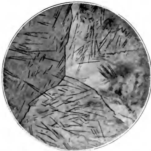
FIG. 22.—Incipient Tourmalinization of Quartz. Three quartz grains shown. Needles single and in bunches of tourmaline, Mount Bischoff Tasmania. (Alfred W. von Fircks, copied by Lindgren in T.A.I.M.E. Vol. XXX, page 637.) Shows how crystals of tourmaline pass from one quartz into the other.
